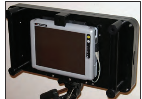
Image D.4: Looking Through Walls radar
