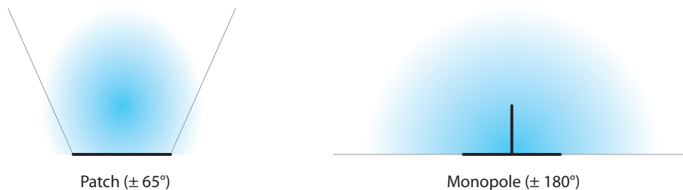
Image 8.5: Patch vs. Monopole angle of reflection. Note that the antenna-patch has a much smaller reflection angle.
